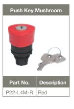
Manual push "In". Automatic latches "In". Turn key clock-wise to release. Spring return. Key withdrawable "Out" position only. Red only.
